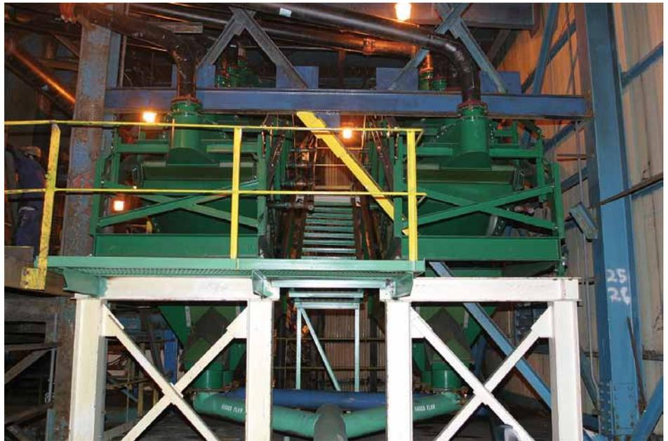
Figure 1. Leatherwood Stack Sizer Installation
