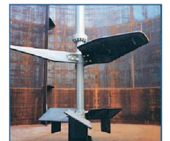
Concentrate Slurry Mixer
